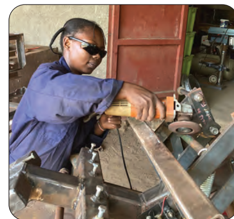
One of Brian Dyck’s team members in South Sudan sanding off the rust in preparation for painting.
