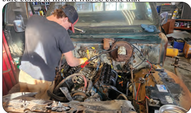
Owen was working on the motor, installing a new manifold, carburetor, valve covers and distributor.
