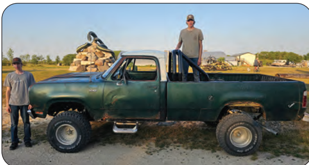
The truck now has a four-inch lift, 33-inch tires and a roll bar to give it that 1980s look. They'll drive it like this for a year or two before they finish the body work and paint it.
