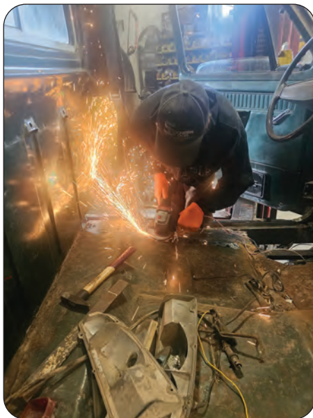
Bohdan working on the floor after the new sheet metal was welded in.
