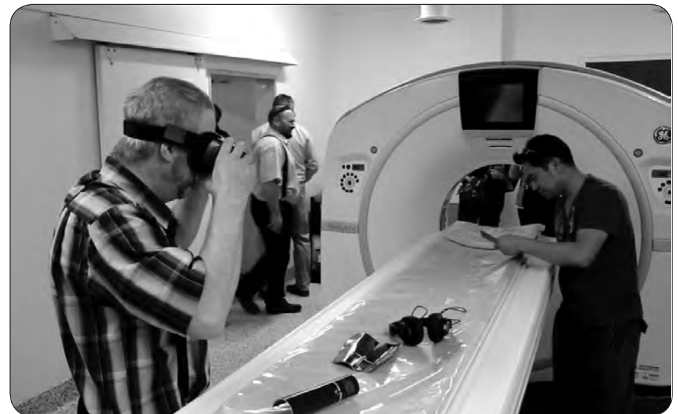
The facility is equipped with a CT scanner for measuring carcass composition, robustness, and meat quality faster and with greater accuracy.
