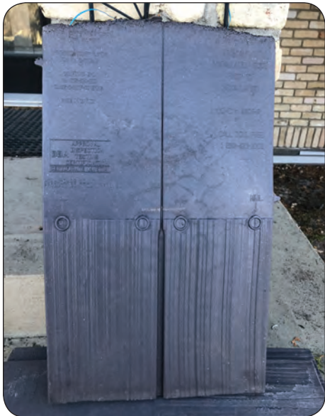
Enviroshake roofing is made from 95 per cent recycled material.
